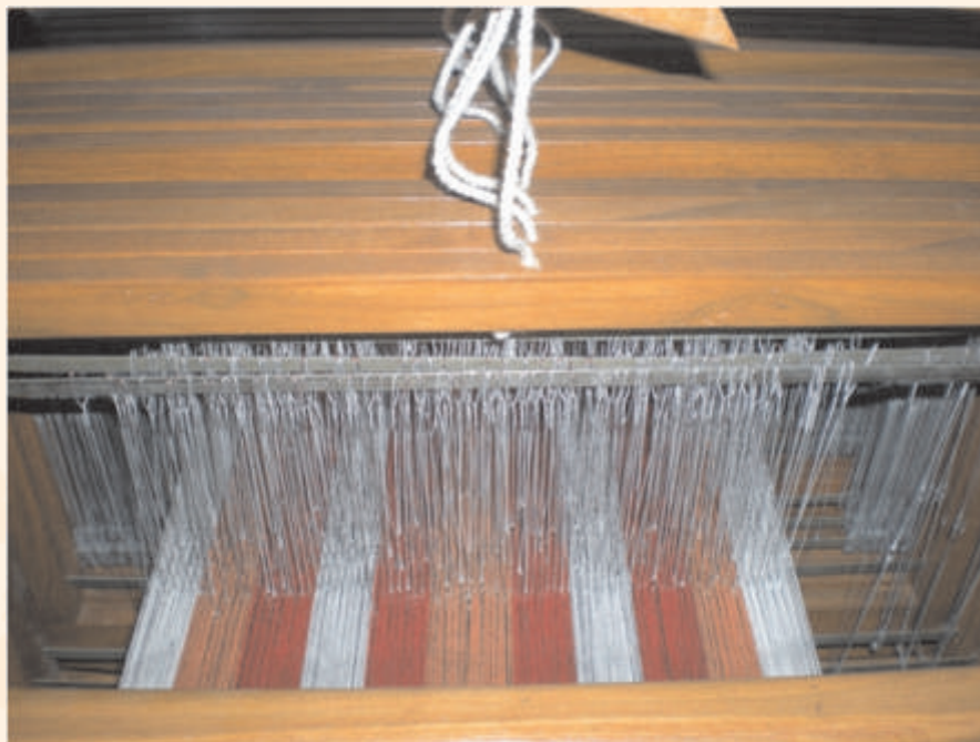
Figure 3.3- The warp yarns through the heald eyes of the heald shafts
