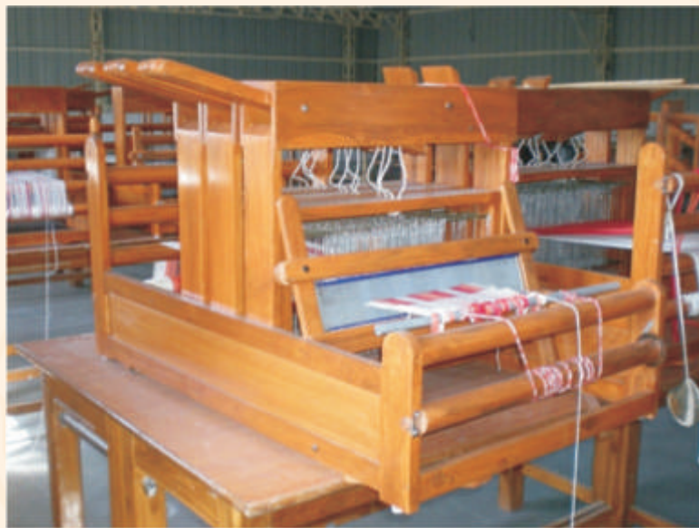
Figure 3.1- Front view of a handloom for weaving sample fabrics
