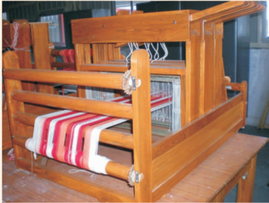
Figure 3.2- Rear view of a handloom for weaving sample fabrics
